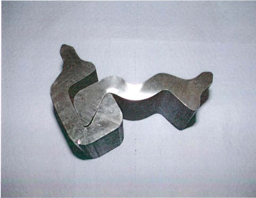
Figure 40: Overview photo, sample no. 16 (LBP100-10), Deformation after test
