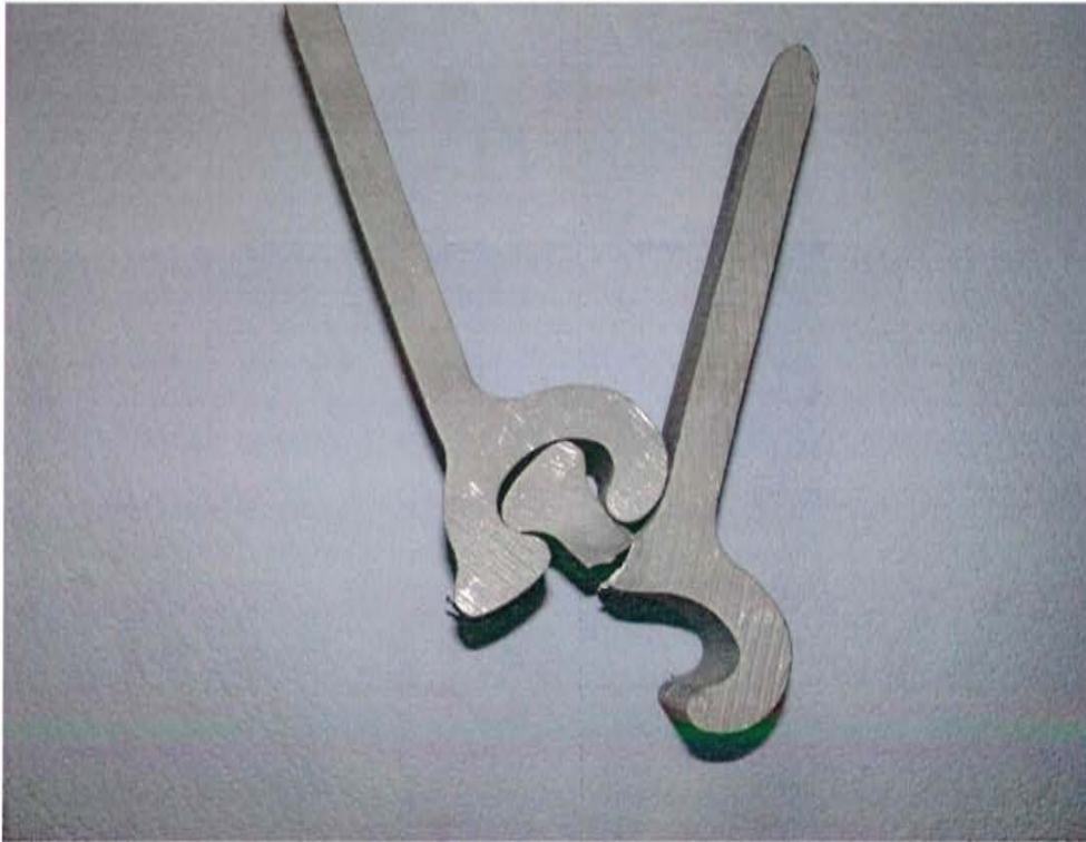
Figure 42: Overview photo, sample no. 20 (FD300-12), Deformation after test
