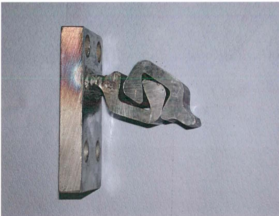
Figure 33: Overview photo, sample no. 15 (LBP100-10), Deformation after test
