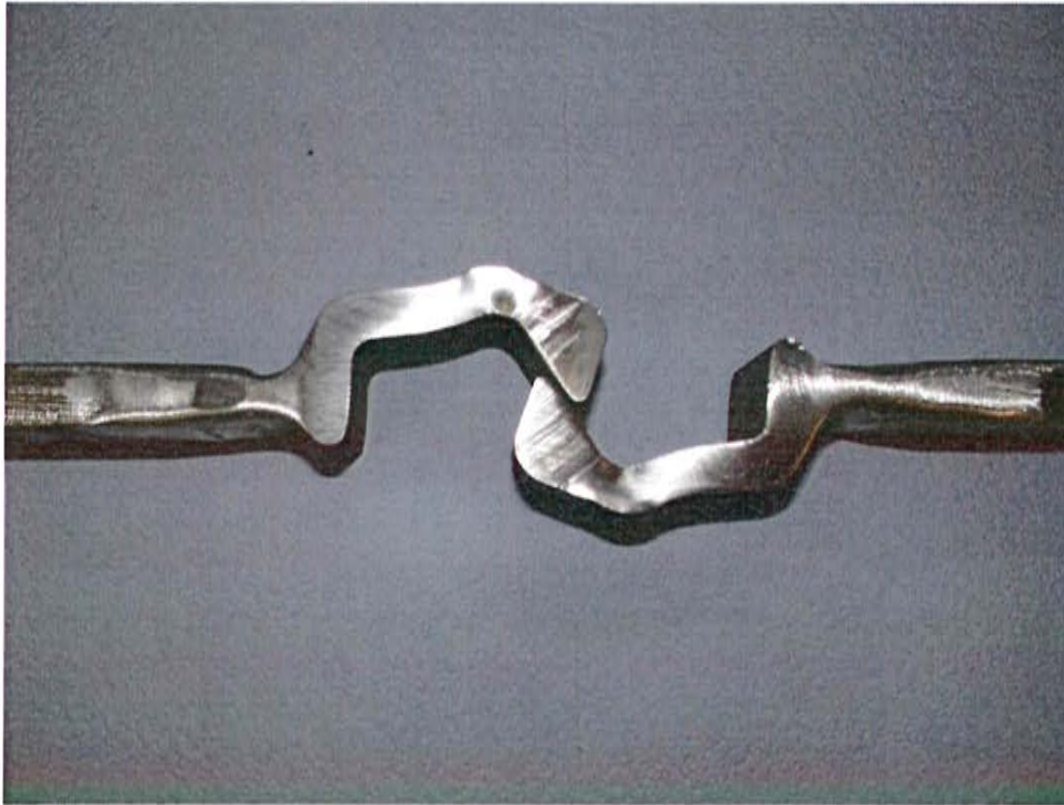
Figure 10: Overview photo, sample no. 14 (LBP100-10), after test, failure by deformation
