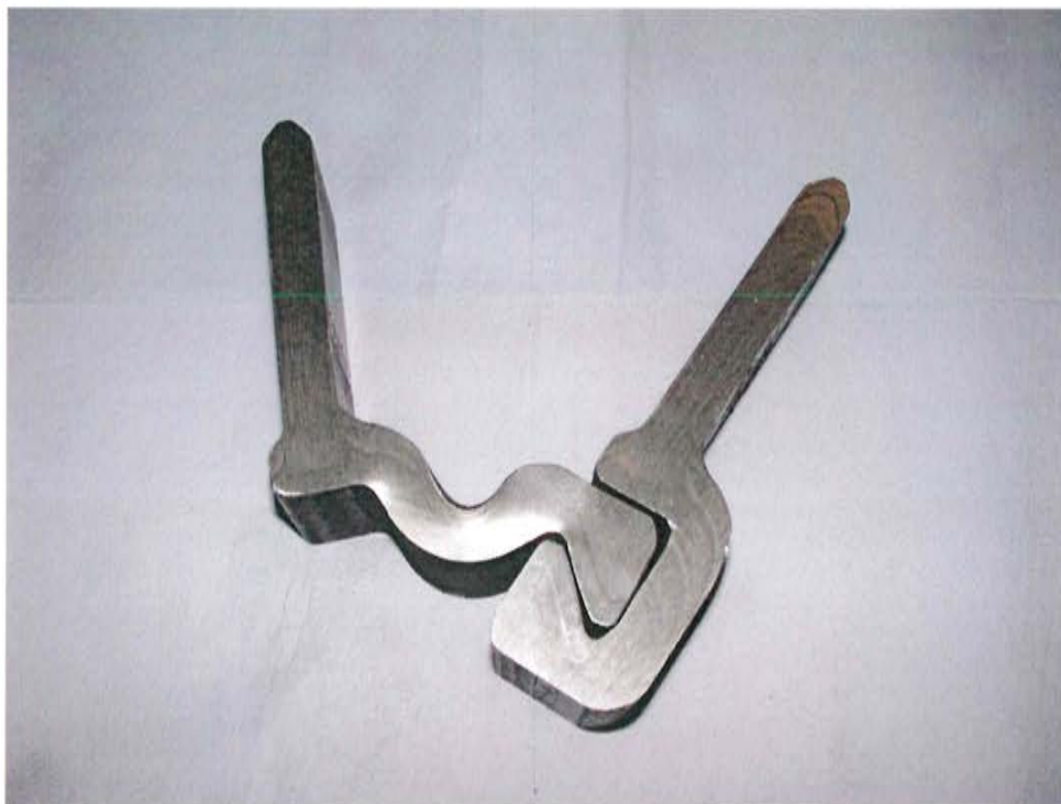
Figure 37: Overview photo, sample no. 6 (LBP300-16), Deformation after test
