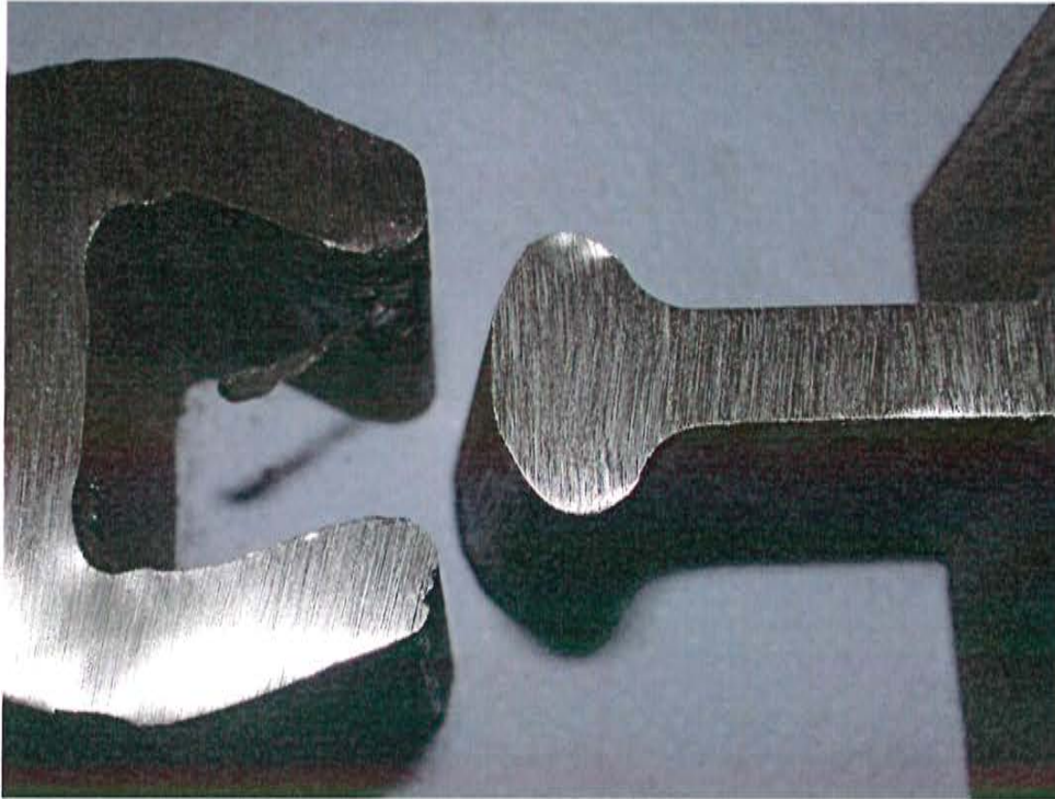
Figure 16: Overview photo, sample no. 21 (PZM/PZF), after test, failure by deformation
