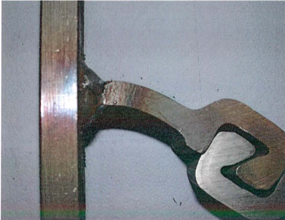
Figure 28: Overview photo, sample no. 9 (LBP180-12), Deformation after test
