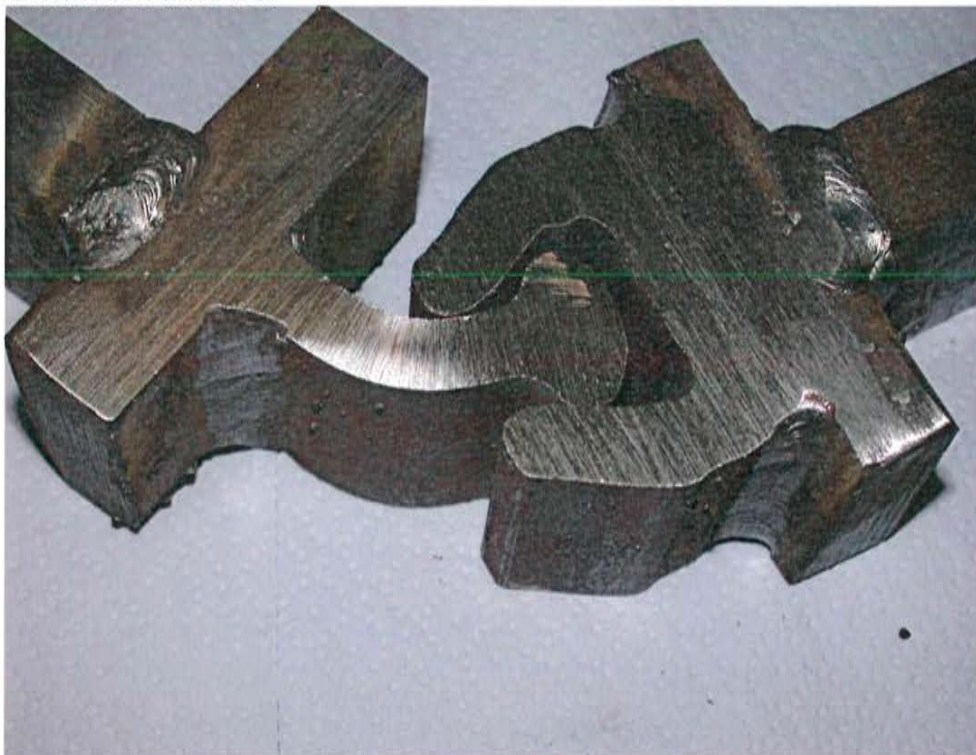
Figure 43: Overview photo, sample no. 22 (PZM/PZF), Deformation after test
