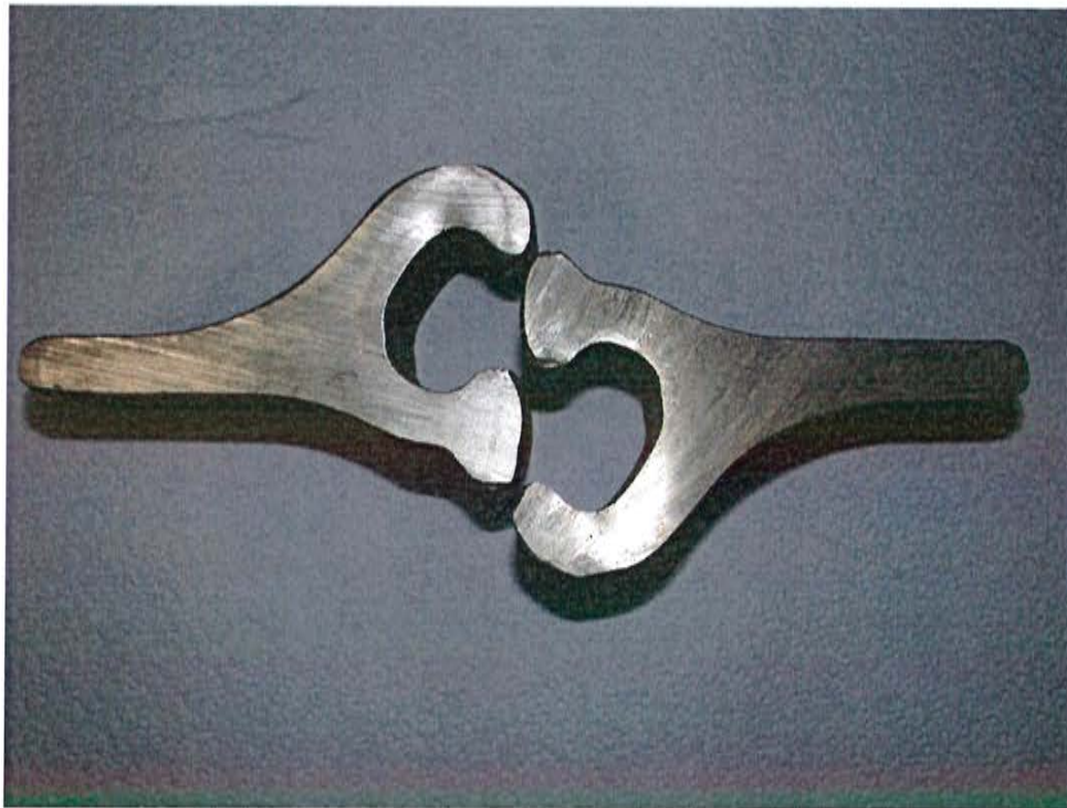
Figure 12: Overview photo, sample no. 17 (FD180-12), after test, failure by deformation
