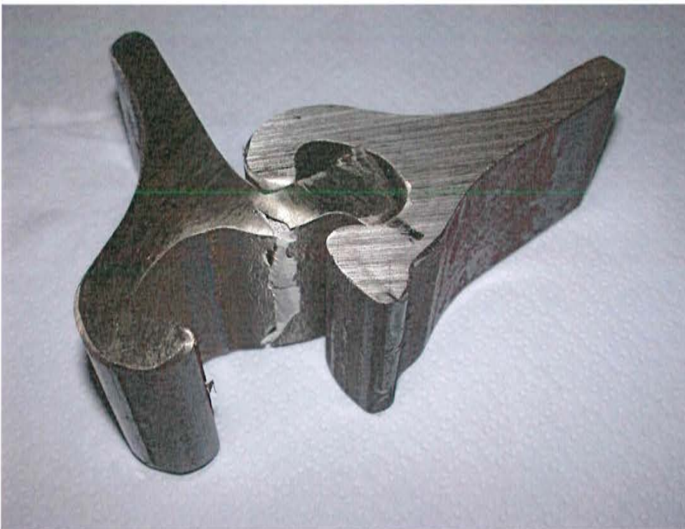
Figure 41: Overview photo, sample no. 18 (FD180-12), Deformation with break after test
